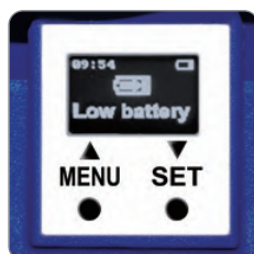
Low Voltage Indicator.
